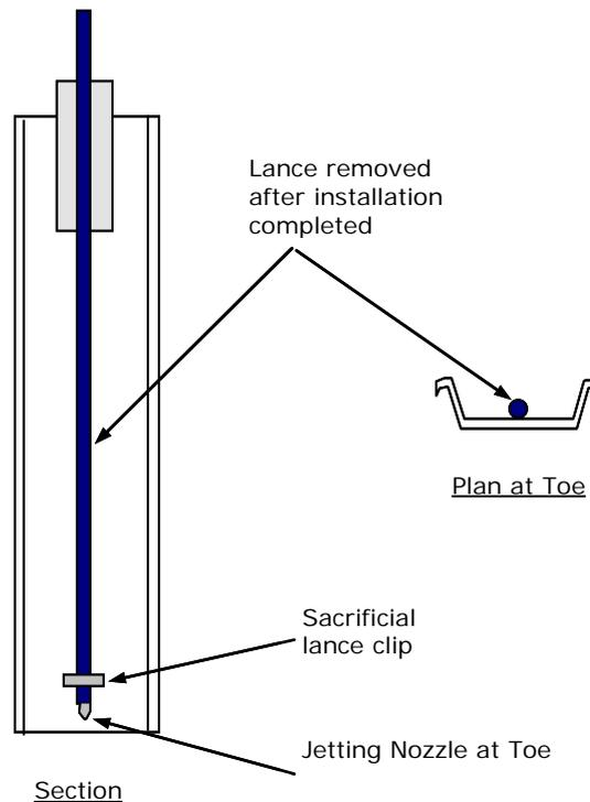
The jet is operated at low pressures in the initial stages of the installation to prevent excessive washout of soil particles. As the installation progresses, the jet is operated continuously throughout the installation to maintain a clear jet nozzle. The water pressure is adjusted in response to the ground resistance to enable the optimum penetration of the pile to be achieved with a minimum disturbance to the structure of the ground.
