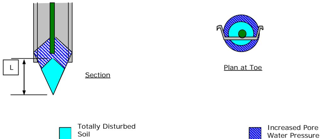
The depth of disturbance 'L' consists of a cone of very high pressure, roughly proportional to that of the jet pressure, within which, the soil structure is totally disturbed. This depth 'L' is a function of the density of the soil and the particle size distribution.
